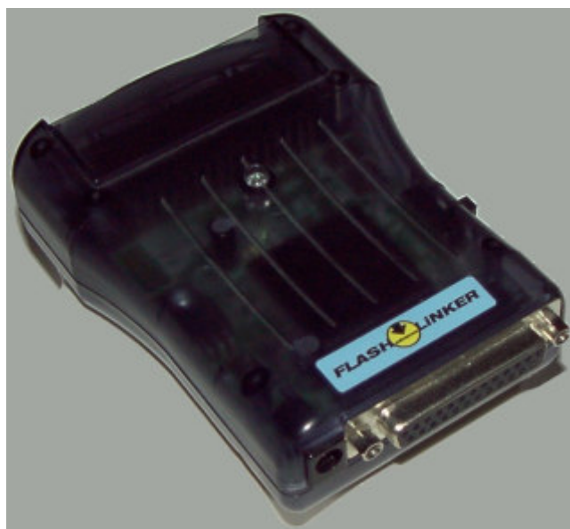
Figure 4.20 The Flash Advance Linker connects to a PC using a parallel port cable.
